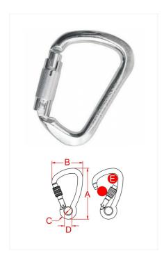
AISI 316 stainless steel connector with Auto Block sleeve. The X-Large is designed to offer a wide gate opening and a high tensile strength. The particular D shape prevents the rotation of the carabiner and allows to distribute the load along the major axis.
