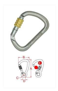
Carbon steel carabiner with screw sleeve. The X-Large is designed to offer a wide gate opening and a high tensile strength. The particular D shape prevents the rotation of the carabiner and allows to distribute the load along the major axis.
