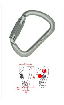
Carbon steel carabiner with Auto Block sleeve. The X-Large is designed to offer a wide gate opening and a high tensile strength. The particular D shape prevents the rotation of the carabiner and allows to distribute the load along the major axis.
